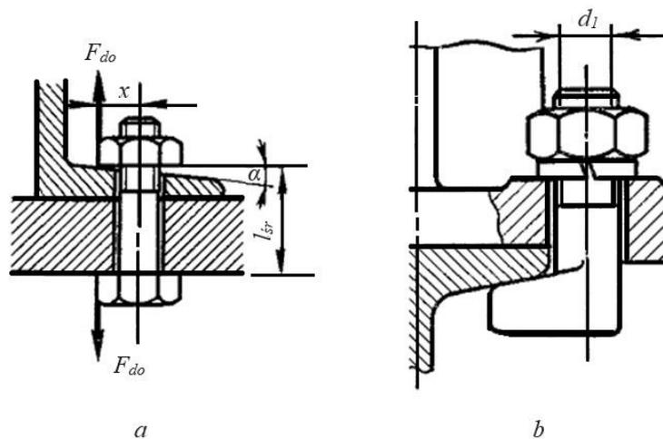
Fig. 3.22. Loading of the joint with centrifugal force
