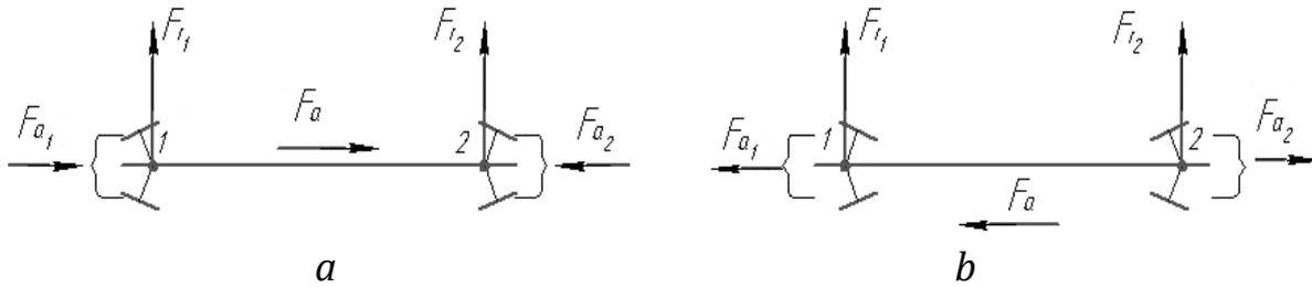
Fig. 3.56. Load patterns for angular contact bearings:
