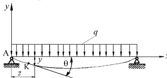
Fig. 2.15. Diagram of forces acting on the beam
