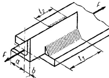
Fig. 3.6. Flange welds in asymmetric member joints loaded with axial force
