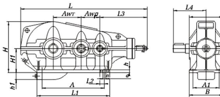
Fig. D.10. Conical-cylindrical three-stage gearboxes type KC2
