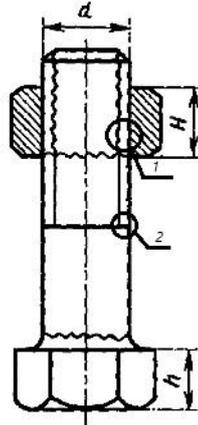
Fig. 3.15. Areas of possible damage to fixing connections
