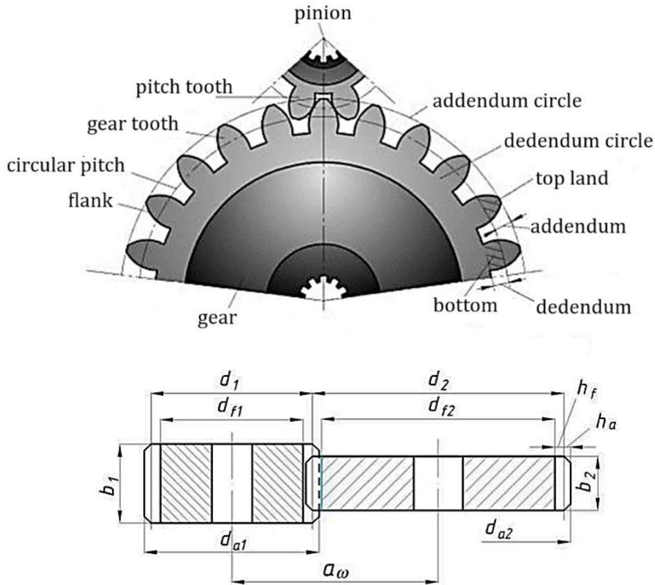
Fig. 3.36. The geometry of a helical gearbox
