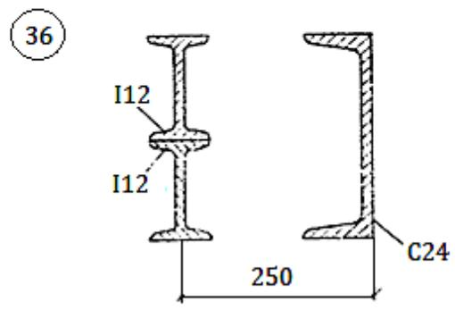
**Task 2.5.** Determine the position of the principal central axes, the values of the principal central moments of inertia and the bending strength indices (see diagram for the task).
