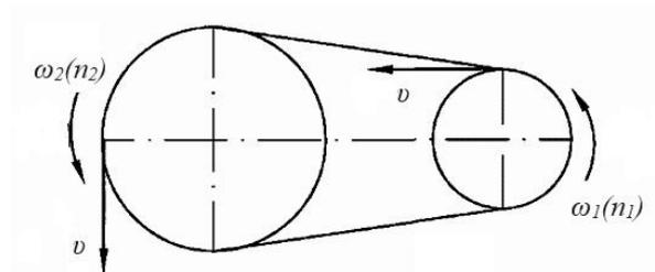
Fig. 3.33. Calculation scheme for the belt transmission to Example 3.21
