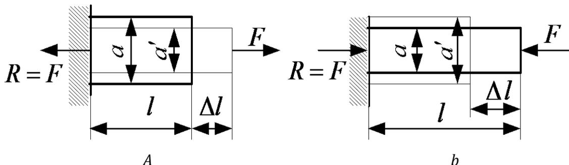
Fig. 2.2. Deformation in uniaxial state of stress:
