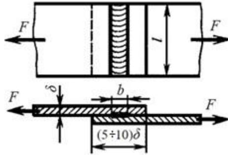
Fig. 3.9. Calculation scheme of continuous contact welding
