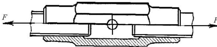
Fig. 3.17. Forces in a threaded connection
