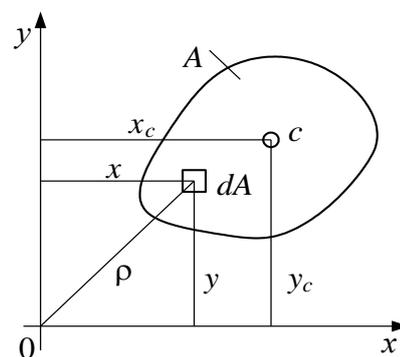
Fig. 2.7. Cross-section of a bar with an  $xy$  system
