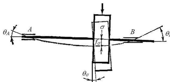
Fig.3.45. Deflection and rotation angles of shaft sections
