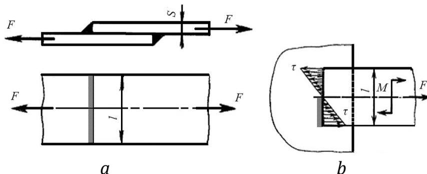
Fig. 3.4 Diagram of forces and moments in an overlap weld: a - loaded with axial force; b - loaded with bending moment
