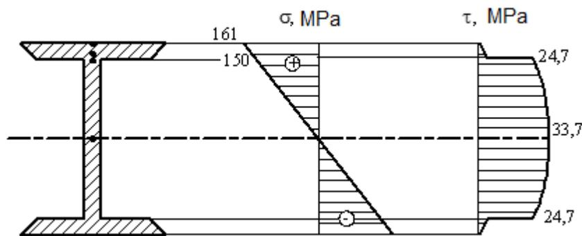
Fig. 2.23. Diagram of normal and tangential stresses in an I-beam
