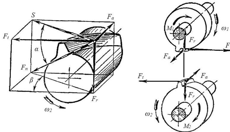
Fig. 3.39. Forces acting in a gear mesh with bevel teeth
