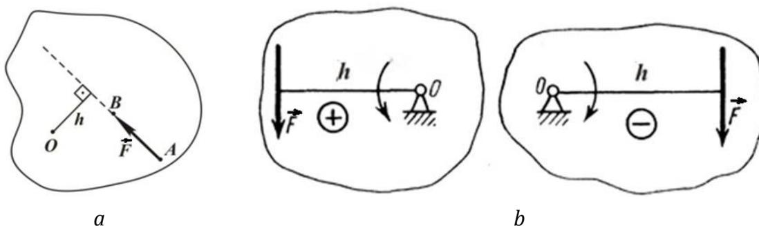
Fig. 1.9. Moment of force relative to a point:
