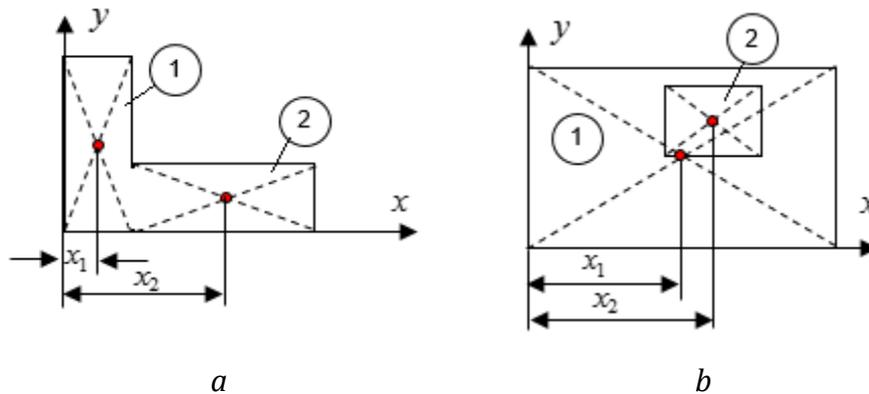
Fig. 1.19. Determination of the centre of gravity of figures:
