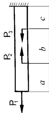
**Task 2.2.** Select the cross-section of the rod holding the crossbar (see the schemes for the calculation). Material - steel S215.
