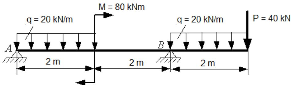
Fig. 2.21. Beam loading scheme
