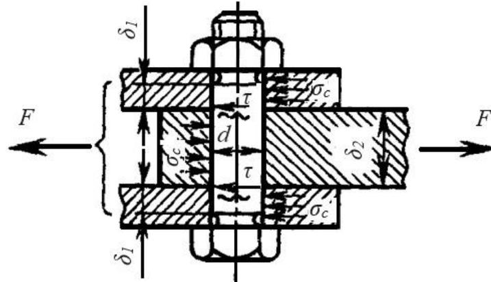
Fig. 3.18. Diagram of the calculation of bolts placed in a hole without a slot
