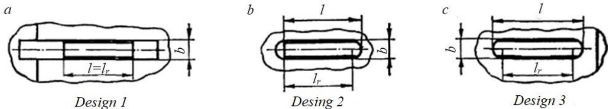
Fig. 3.28. Basic types of prismatic inlets
