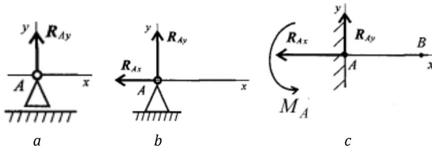
Fig. 1.13. Determination of reactions in supports:
