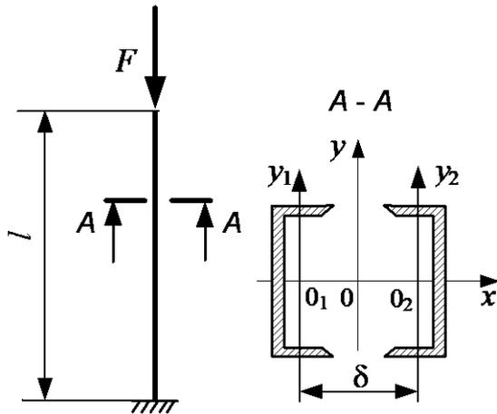
Fig. 2.31. Column scheme to Example 2.18
