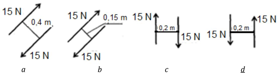
Fig. 1.10. Variants for defining a pair of equivalent forces
