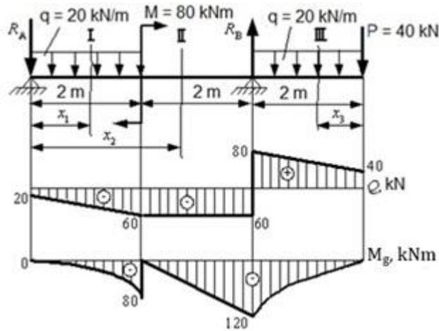
Fig. 2.22. Diagram of shear forces and bending moments for the beam of Example 2.14
