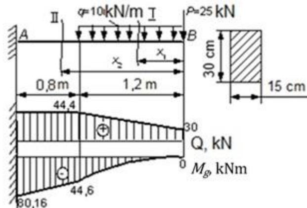
Fig. 2.20. Beam loading scheme
