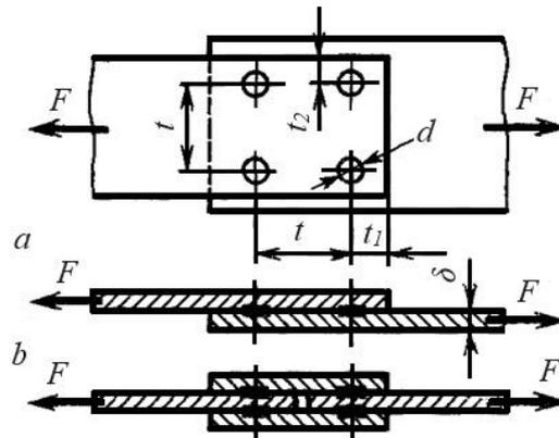
Fig. 3.8. Diagram of spot welding calculations:
