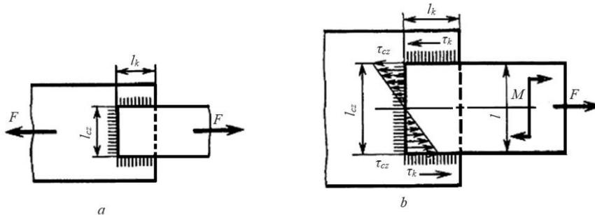
Fig. 3.5. Distribution of forces in combined welds:
