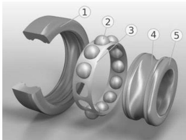
Fig. 3.55. Rolling bearing
