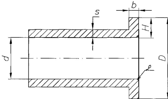
Fig. 3.51. Diagram for determining the dimensions of a flanged insert
