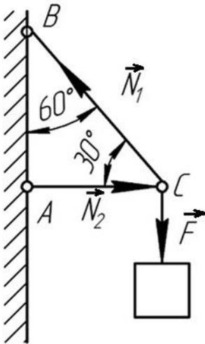
Fig. 1.2. Reactions forces in bars
