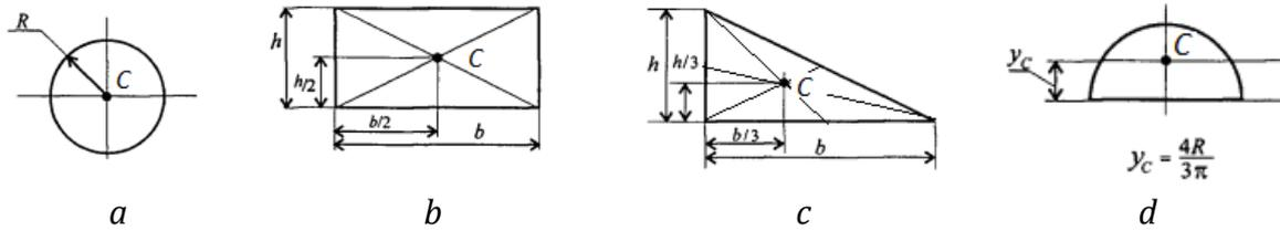
Fig. 1.17. Position of the centres of gravity of the figures:
