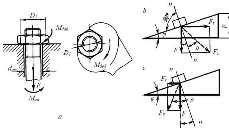
Fig. 3.13. Interaction forces between bolt and nut
