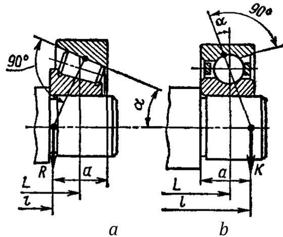
Fig. 3.57. Diagram for calculating the addition points of the angular contact bearing support reactions: *a* - "stripping" scheme; *b* - "extending" scheme
