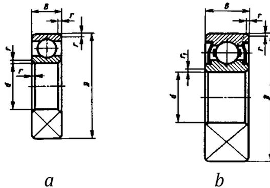
Fig. D.11. Single row radial ball bearings:
