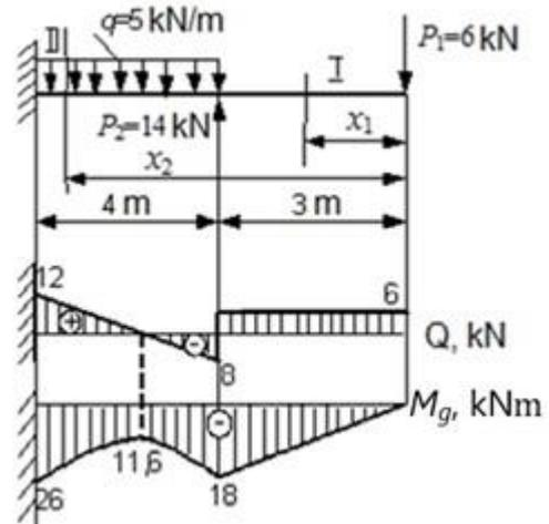
Fig. 2.18. Beam loading scheme
