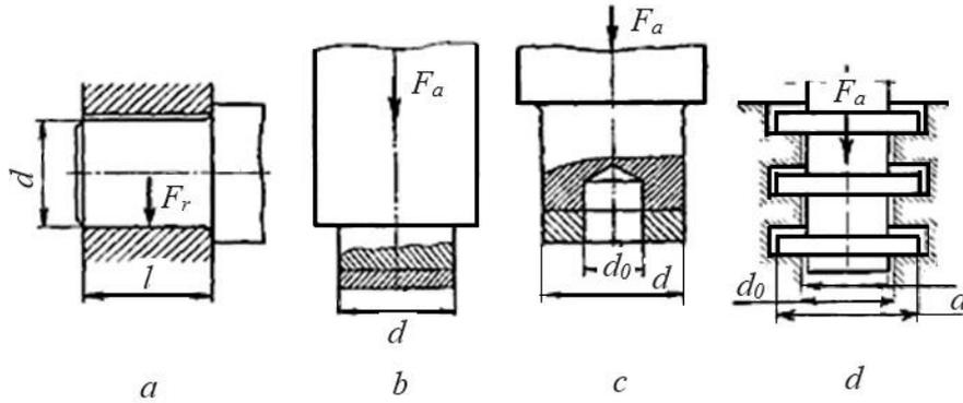
Fig. 3.50. Diagram of occurrence of forces in sliding bearings with imperfect lubrication:
