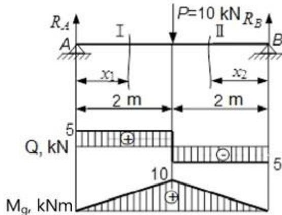
Fig. 2.16. Beam loading scheme
