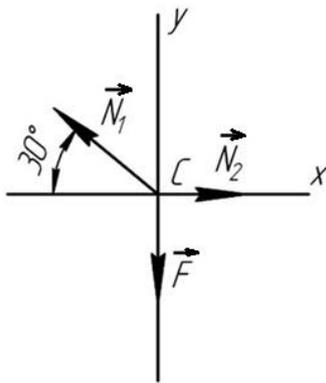
Fig. 1.3. Force distribution in the implemented coordinate system
