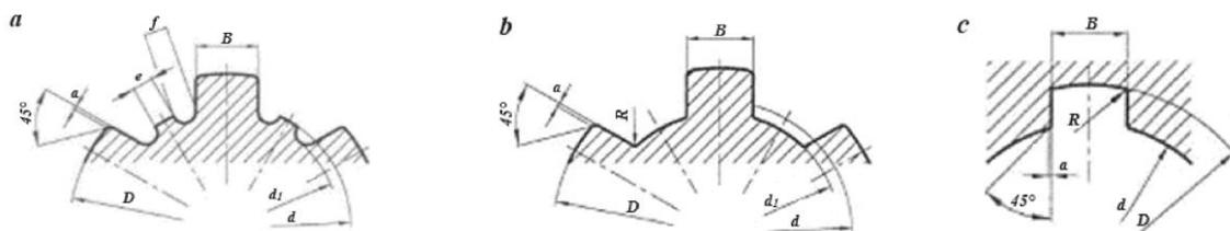
Fig. D.4. Parallel spline connections (PN-M 85017):
