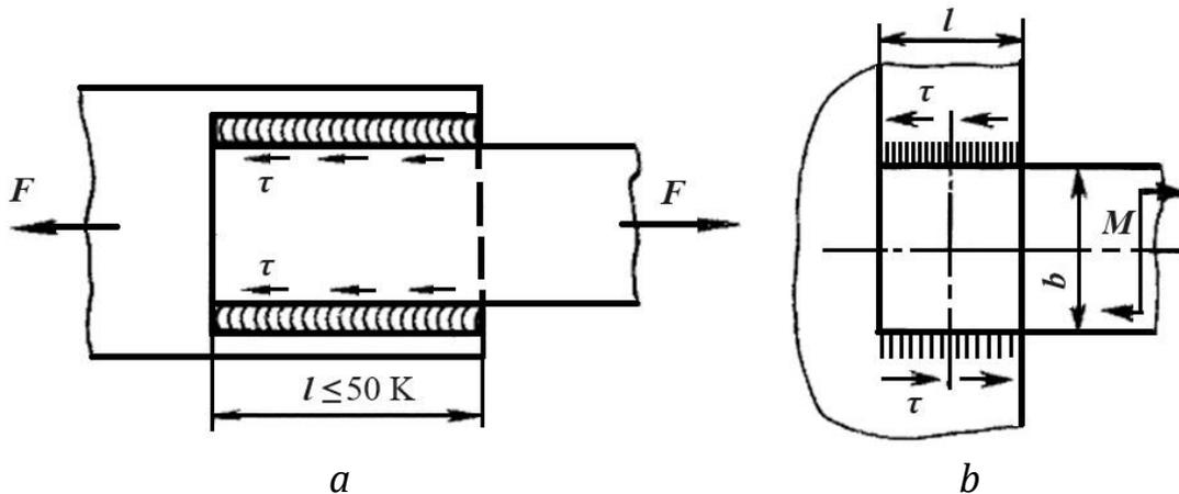
Fig. 3.3. Forces occurring in a flange weld:
