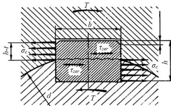
Fig. 3.27. Calculation diagram for a prismatic keyway connection
