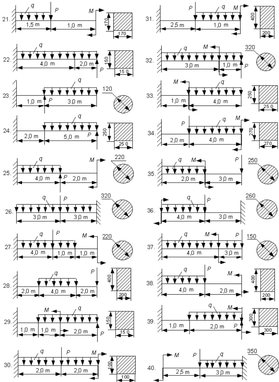
**Task 2.8.** Based on the strength and stiffness criteria, select the cross-section of the beam (calculation schemes).
