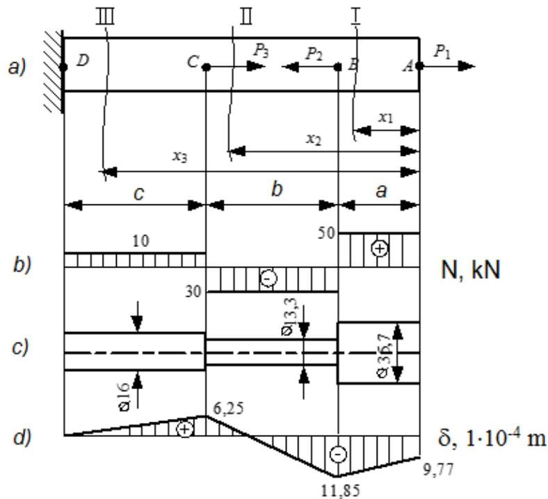
Fig. 2.3. Diagram of the bar to Example 2.1:
