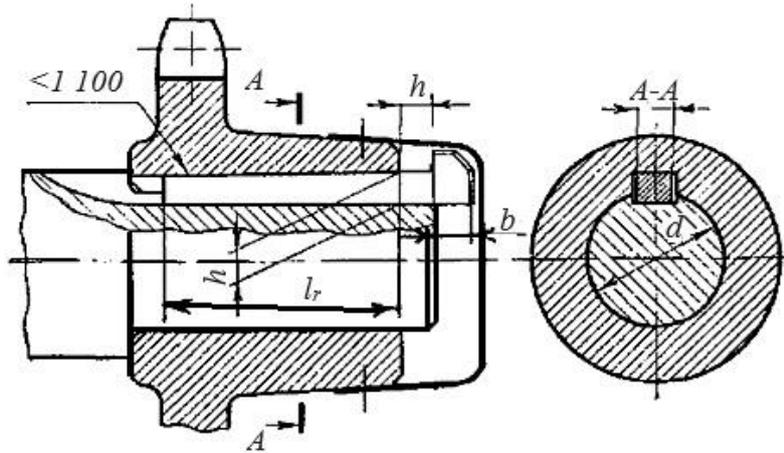
Fig. 3.24. Prismatic key connection
