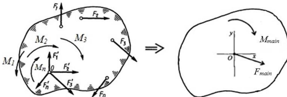
Fig. 1.12. The main torque of the system
