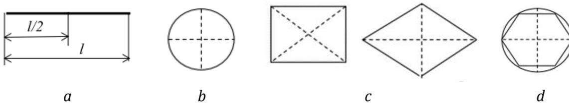
Fig. 1.18. The centre of gravity of:
