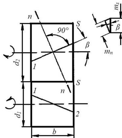
Fig. 3.37. Schematic diagram of a gearbox with oblique teeth
