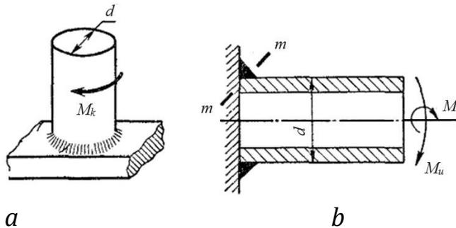
Fig. 3.7. Calculation scheme of a fillet weld:
