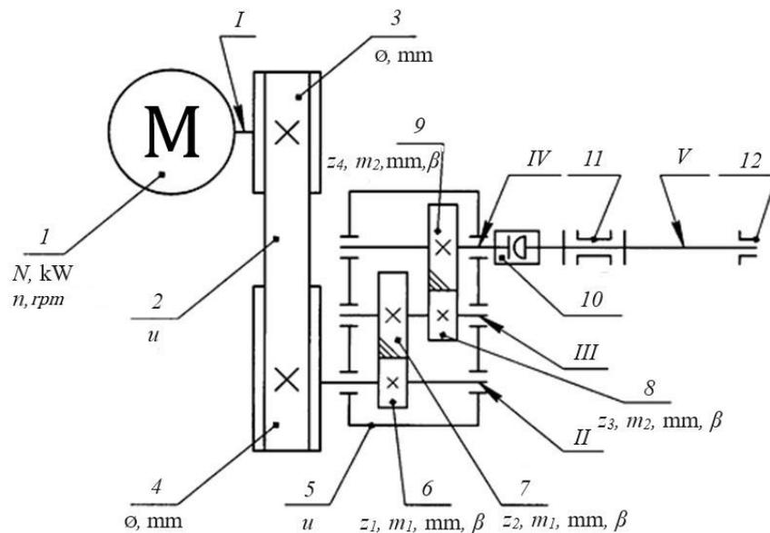
Fig. 3.43. Kinematic diagram of the drive:
