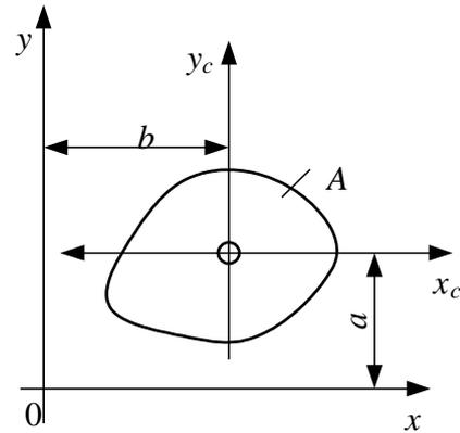
Fig. 2.8. Cross-section of a bar with an  $xy$  system
