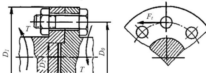
Fig. 3.21. Diagram of a torque loaded threaded connection
