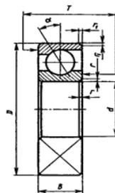
Fig. D.12. Single row radial thrust ball bearings (ISO 492:2014)
