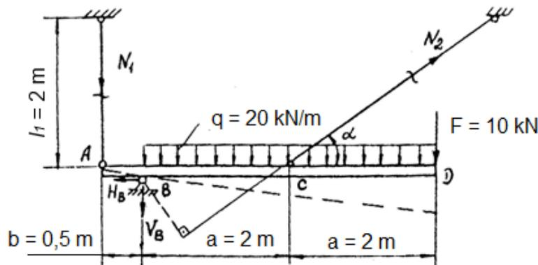
Fig. 2.5. Diagram of a statically indeterminate bar system to Example 2.3
