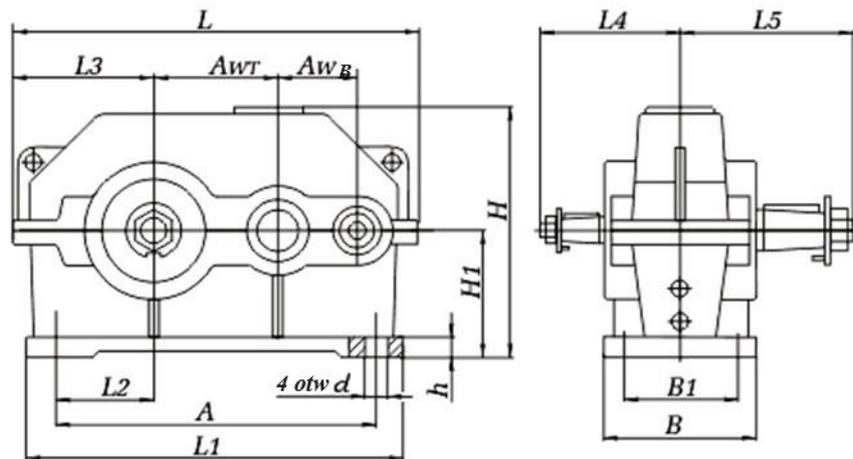
Fig. D.7. Cylindrical two-stage transmission 1C2U
