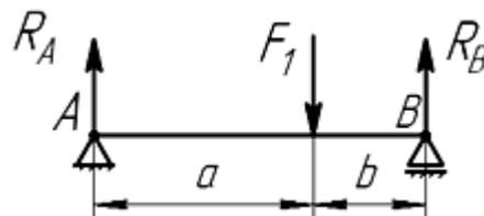
Fig. 3.48. Diagram of forces acting on the axle
