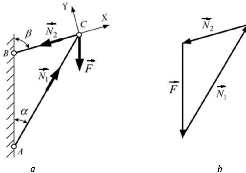
Fig. 1.6. Bracket: a - distribution of forces in the bracket; b - force triangle
