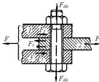
Fig. 3.19. Diagram for calculating bolts in clearance holes
