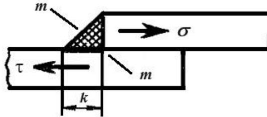
Fig. 3.2. Diagram of a fillet weld and the forces involved
