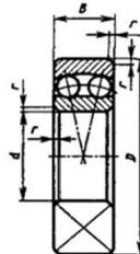
Fig. D.12. Radial spherical double-row ball bearings (ISO 15:1998)
