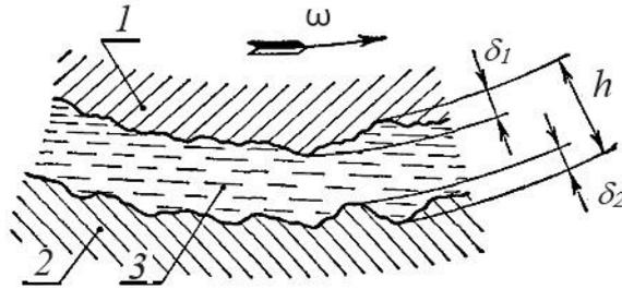
Fig. 3.49. For calculation of the fluid friction mode:
