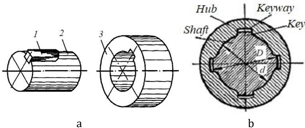
Fig. 3.23. Keyed (a) and splined (b) connections
