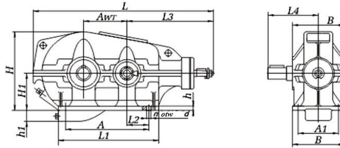
Fig. D.9. Two-stage bevel-cylinder gearboxes of type KC1
