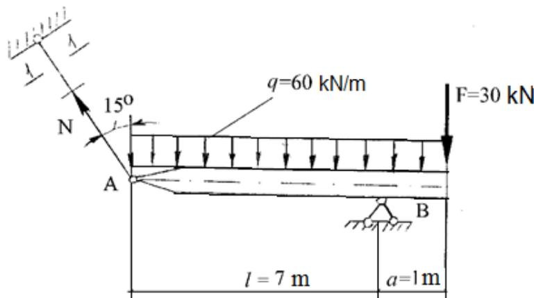
Fig. 2.4. Forces acting on the beam to Example 2.2
