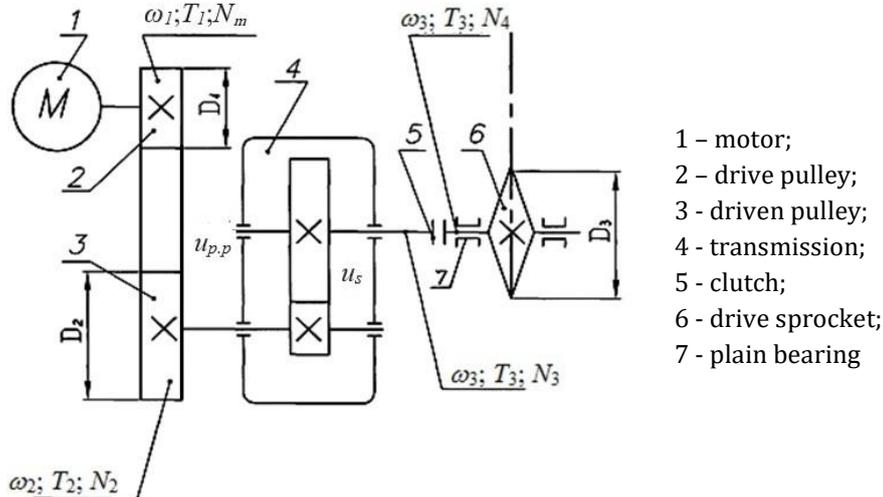
Fig. 3.34. Kinematic diagram of a chain conveyor drive
