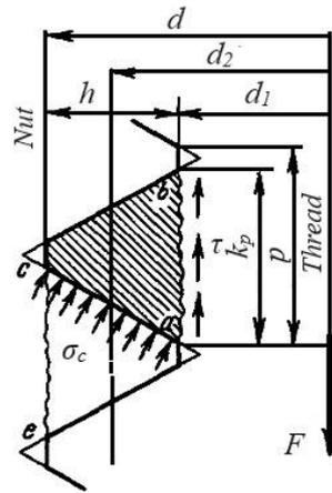
Fig. 3.14. Force diagram for calculating thread strength and wear resistance
