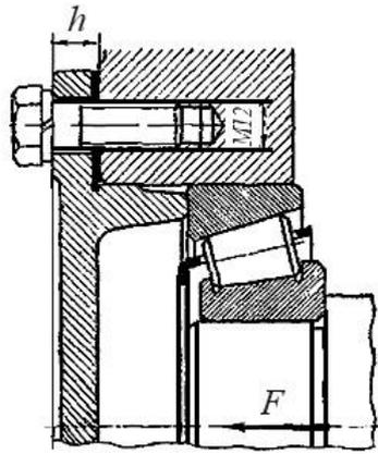
Fig. 3.20. Strength distribution of the tightened connection
