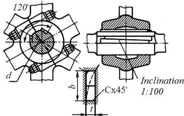
Fig. 3.26. Tangential groove connection
