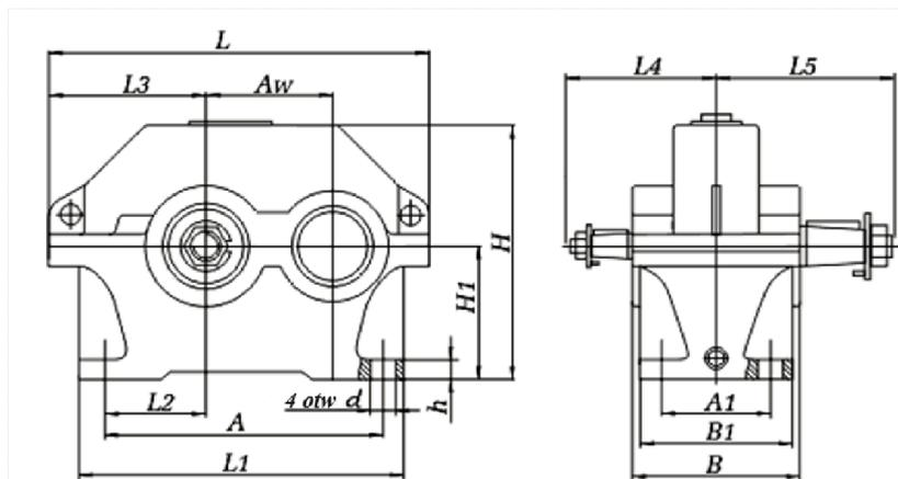
Fig. D.6. Single-stage cylindrical gear 1CU
