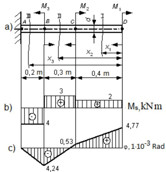
Fig. 2.12. Rod diagram to Example 2.7: a - load diagram; b - diagram of torsional moments; c - diagram of torsion angles of beam sections
