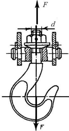
Fig. 3.16. Diagram of forces in a thread loaded with an axial force
