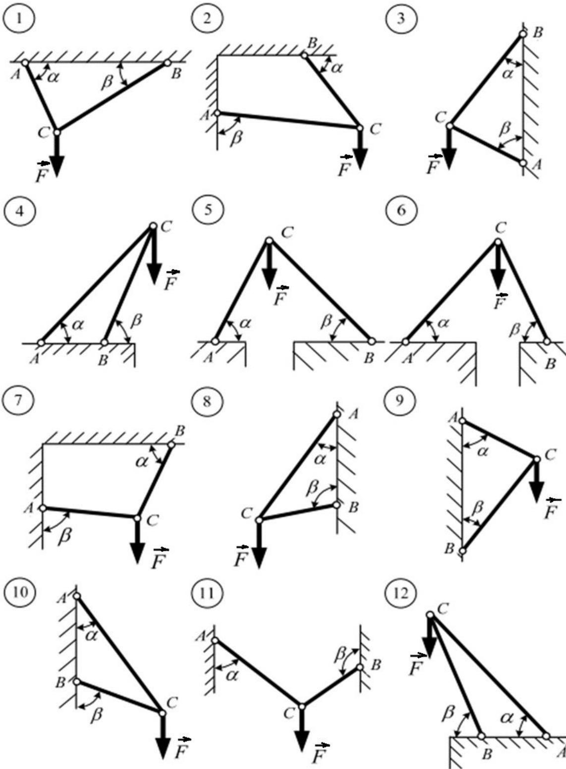
**Task 1.2.** Determine the values and direction of the node reactions for the schemes shown below. The data for the task is shown in Table 1.2.
