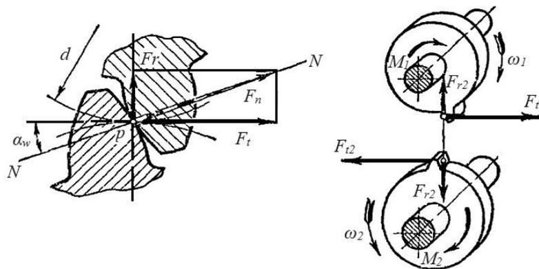
Fig. 3.38. Forces acting in a straight helical gear mesh
