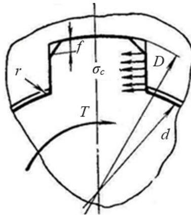
Fig. 3.30. Calculation scheme for spline connections
