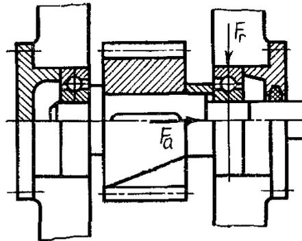
Fig. 3.58. Bevel gear reduction gearbox
