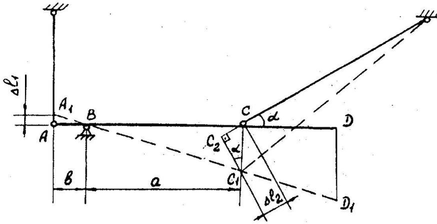
Fig. 2.6. Deformed state of the system
