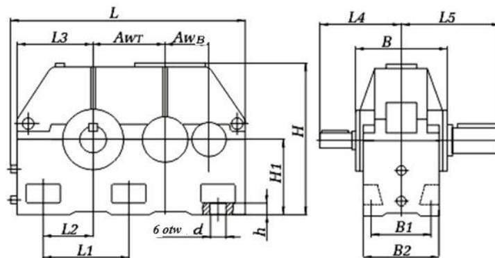
Fig. D8. Cylindrical two-stage gearboxes 1C2Y, 1C2N
