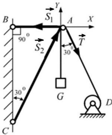
Fig. 1.7. Force distribution in the calculated system
