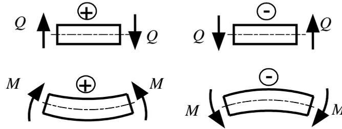
Fig. 2.14. Principle of determining forces and bending moments
