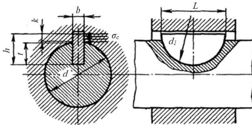
Fig. 3.29. Calculation diagram for shuttle keyway connection
