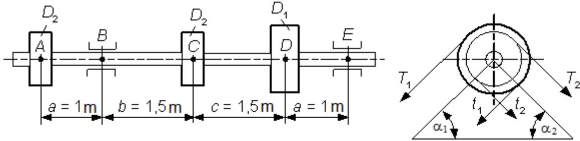
Fig. 2.25. Schematic of the drive shaft
