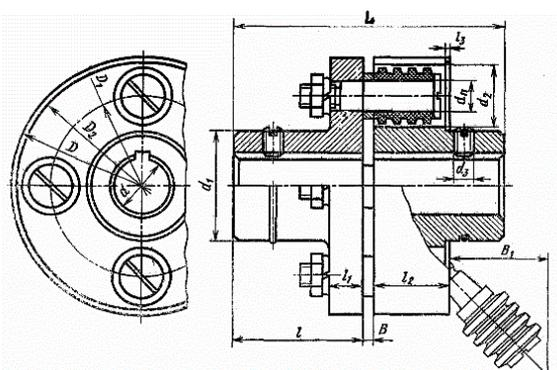
Fig. D.13. Sleeve-finger spring coupling (ISO-R775)
