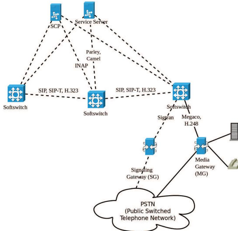
FIGURE 3. The NGN application level built according to the principle of centralized control
