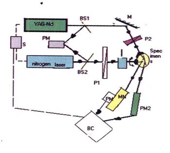
**Fig. 1.** Experimental setup for performing the photoinducing nonlinear optical measurements
