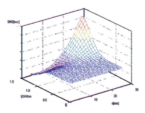
**Fig. 1.** Dependence of the photoinduced SHG versus the photoinducing beam power I and the fiber diameter d at T=149 K
